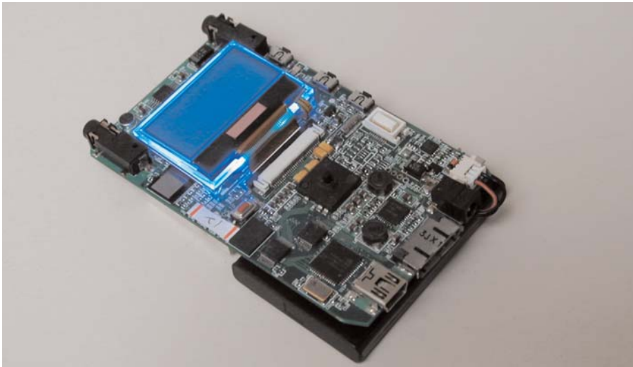
MCF5249 based MP3 player, recorder & FM radio running Freescale's TRIO digital audio software built with the Crossware version 4.0 ColdFire C/C++ compiler.
