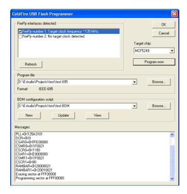
Windows flash programming software is included. This can simultaneously control up to 127 FireFly devices, programming any or all of the target boards connected to them.
